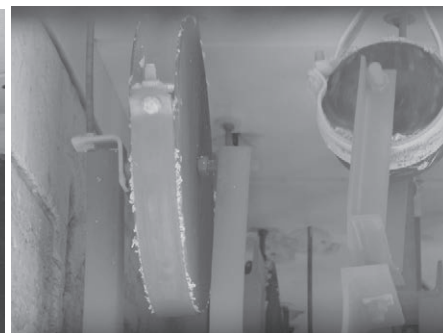
Fig. 4: Systems after 90 min. (approx. 1,000 °C)
